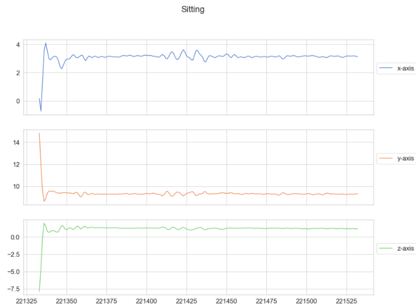
Figure 2 - Three-axis accelerometer plot labeled as sitting after filtering using a third-order 4 Hz Butterworth filter
