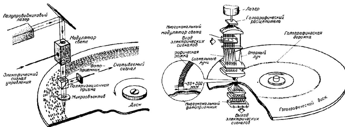
This amount of information can be written down due to a decrease in the size of the holes on the layer and an increase in their number, respectively. The record is produced by Ray in the 700 nm, and read only 440 nm.
