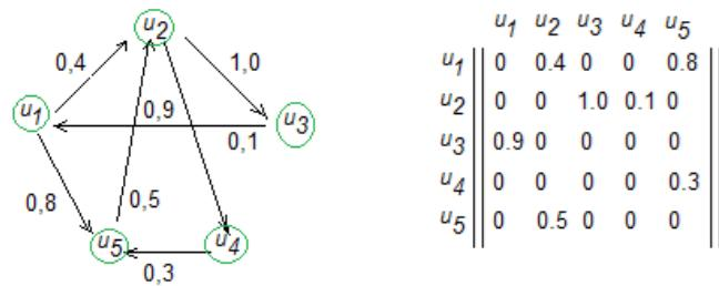
Рис. 1 – Figure 1 - Ratio graph and adjacency matrix  $M_f$  of a fuzzy relation
